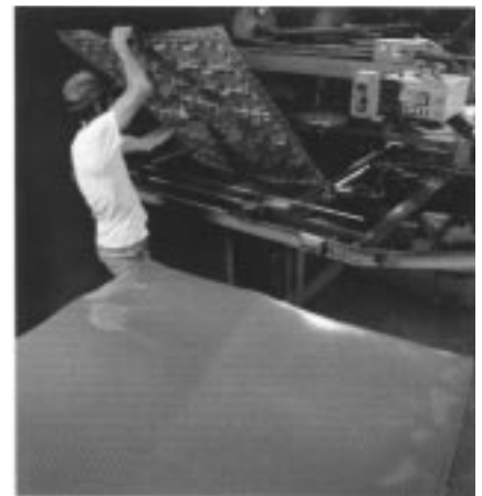
Machine operator removes a thermoformed shipping container for rectangular automobile headlights from a rotary vacuum press.
